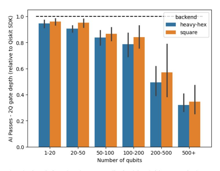
Circuit depth for circuits transpiled with Qiskit+AI, relative to standard Qiskit, for the Benchpress circuits (lower is better)
