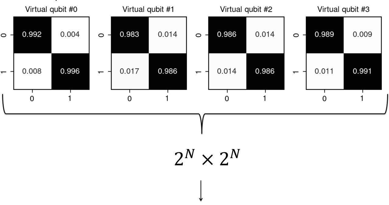
The inverse of the transfer matrix can be used for error mitigation, but it cannot be obtained efficiently in general!
