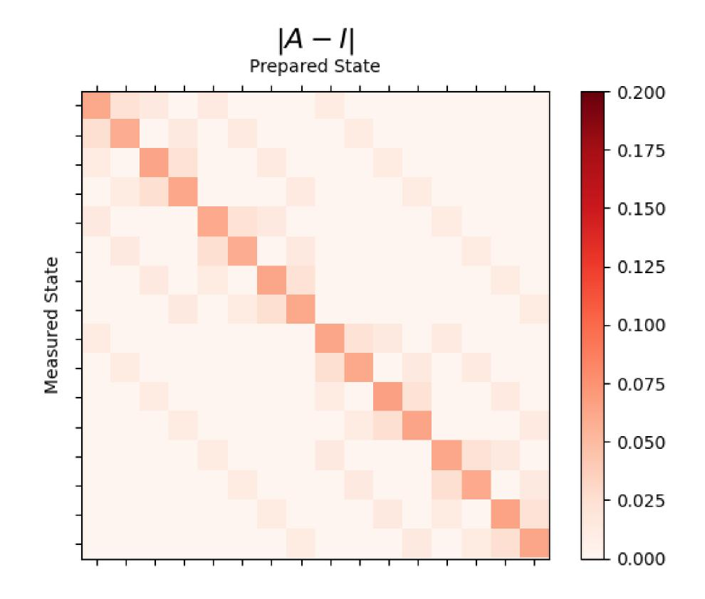
Readouts errors cause the wrong states to be measured.
