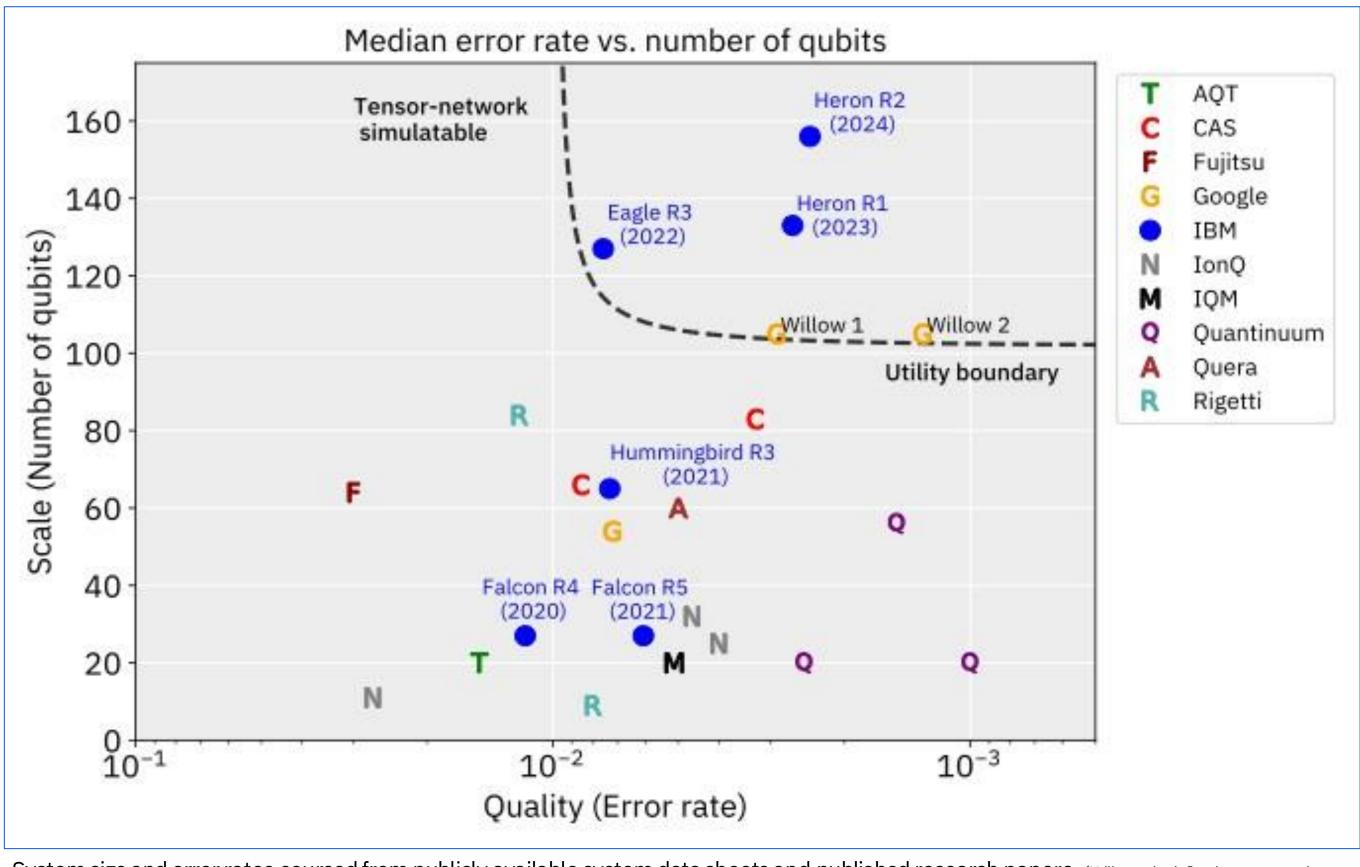
. System size and error rates sourced from publicly available system data sheets and published research papers. (Utility scale defined as proven to be able to run a circuit larger than can be simulated classically by brute-force)
