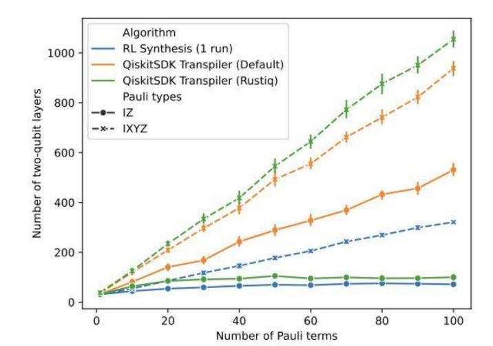
We extend our earlier work on RL-based synthesis of Clifford circuits to general Pauli Networks. We obtain reduction in circuit depth of around 20% on average, and in many cases over 40%.
