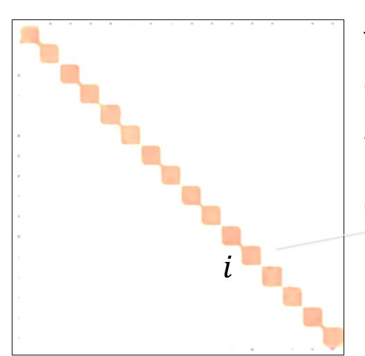
Then, we need to run calibration circuits to get the inverse of the (diagonal) readout error transfer matrix.
