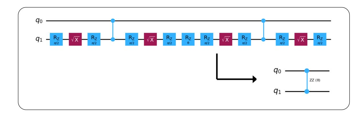
In June: modifications to improve the performance of dynamic circuits, through compression of circuit duration with parallel execution of conditional blocks
