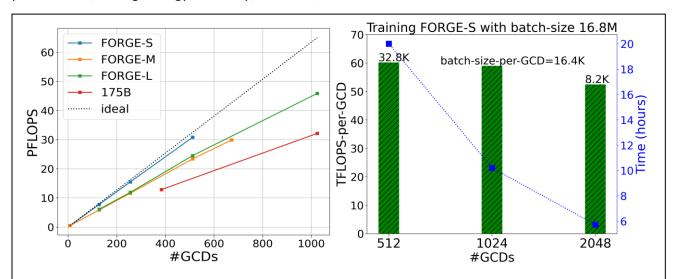
The scaling of both the computation performance (TFLOPS per GCD and aggregated PFLOPS) and time-to-solution (hours) for FORGE models on Frontier. FORGE-M is 13B model.
