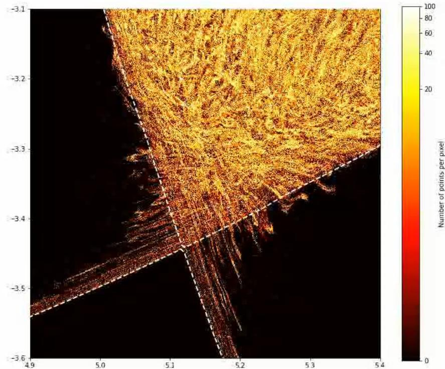
Poincaré puncture plot of magnetic field lines in ITER edge, making the separatrix magnetic surface to be stochastically tangled up by the intrinsic EM turbulence, with thin and long lobes connecting core and divertor plasmas.
