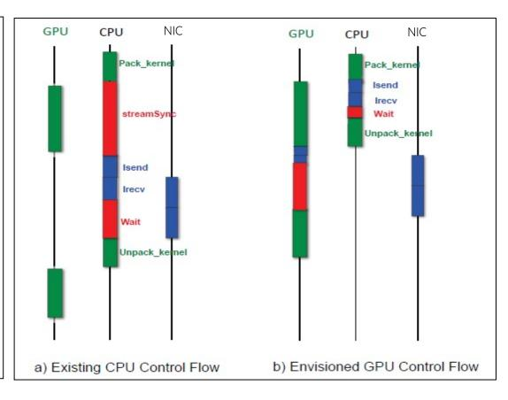
Minimizes CPU – GPU synchronization overheads, communication still occurs at kernel boundary
