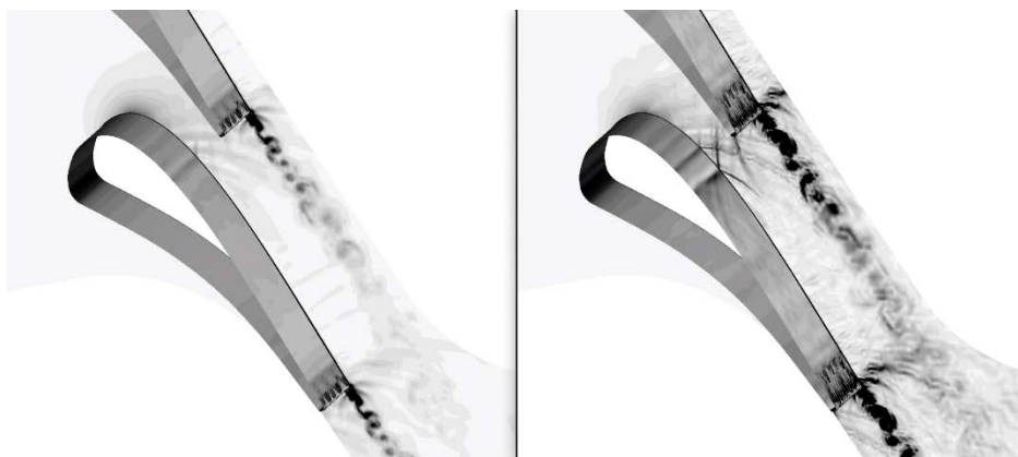
Figure 8.10. GE's GENESIS solver (right) preserves many more wake details of interest in the flow field compared with a commercial solver (left). Image Credit: University of Kansas.
