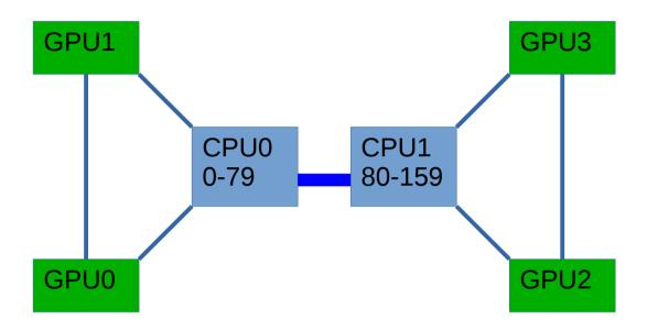
Each CPU socket has 10 cores, 80 hardware threads.
