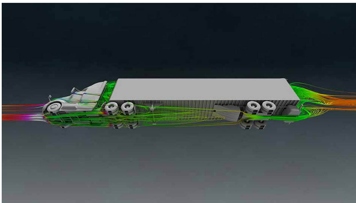
Supercomputing simulations at ORNL enabled SmartTruck engineers to develop the UnderTray System, some components of which are shown here. The system dramatically reduces drag—and increases fuel mileage—in long-haul trucks. Image credit: Michael Matheson, ORNL
