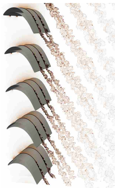
Figure 3.1. A simulation of flow over five jet engine low-pressure turbine blades. Credit: Vincent Lab, Imperial College.
