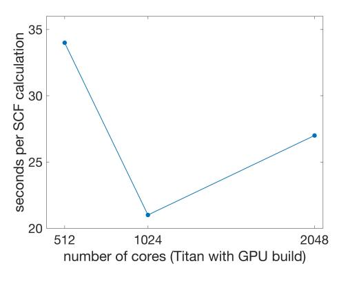
CP2K employs heavy use of scientific libraries like scalapack, fftw, and blacs, and performs well on hyper-threaded Intel Xeons, and when MKL with threaded fftw and blacs is available. Currently the GPU portion of the code seems to improve the performance and scaling less, for smaller (large) systems
