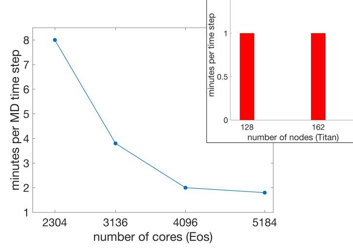
Actual production settings, 623 atom ribonucleotide system with 300 explicit waters, CP2K MD with linear-scaling SCF, using PBE, the D3 dispersion correction, a 400 Ry PW cutoff, DZVP, SCF cutoff 1E-5 and filter cutoff 1E-6, A: Titan, B; Eos, and 2207 atom tetranucleotide system with same settings, C and D. Cores used with D were 1024 and 1296, because the GPU build does not permit use of more than 8 cores per node.
