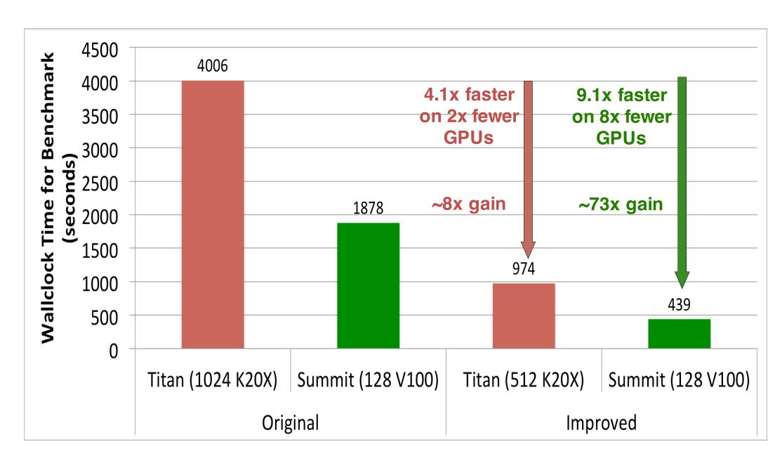
Trajectory times for a benchmark on Summit and Titan showing overall gains. Due to the power of 2 problem size, only 4 out of 6 GPUs were used on Summit nodes.
