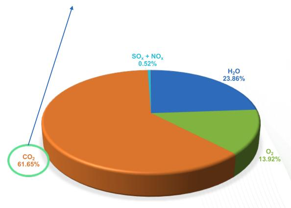
Non-N<sub>2</sub> flue gas components
