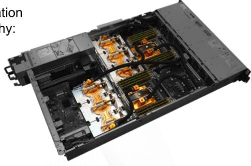
One of Summit's 4,600 IBM AC922 nodes. Each node contains six NVIDIA Volta GPUs and two IBM Power9 CPUs, giving scientists new opportunities to automate, accelerate and drive understanding using artificial intelligence techniques.
