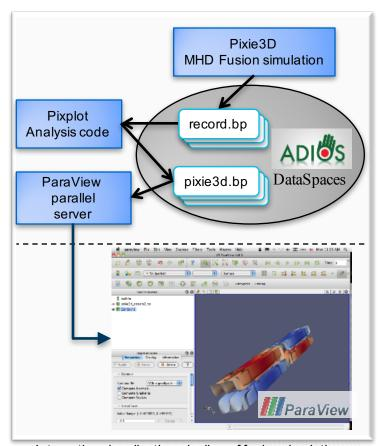
Interactive visualization pipeline of fusion simulation, analysis code and parallel viz. tool
