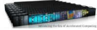
Titan (Cray): Cray XK7 AMD Opteron 6274 16C 2.2 GHz Cray Gemini NVIDIA K20x
