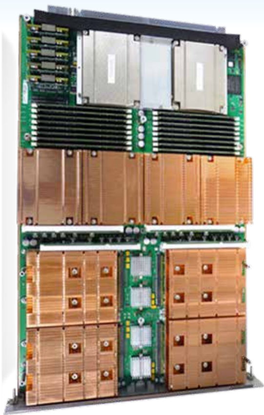
The accelerator-based compute blade used in Titan.
