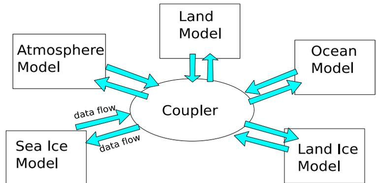
*Integrated Climate Modeling Workflow (based on coupler)*
