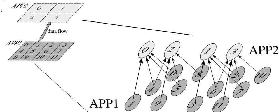
*Tightly Coupled Two-Apps Workflow (based on direct parallel transfer)*
