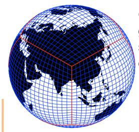
Cubed-sphere grid of CAM spectral element model. Each cube panel is divided into elements.
