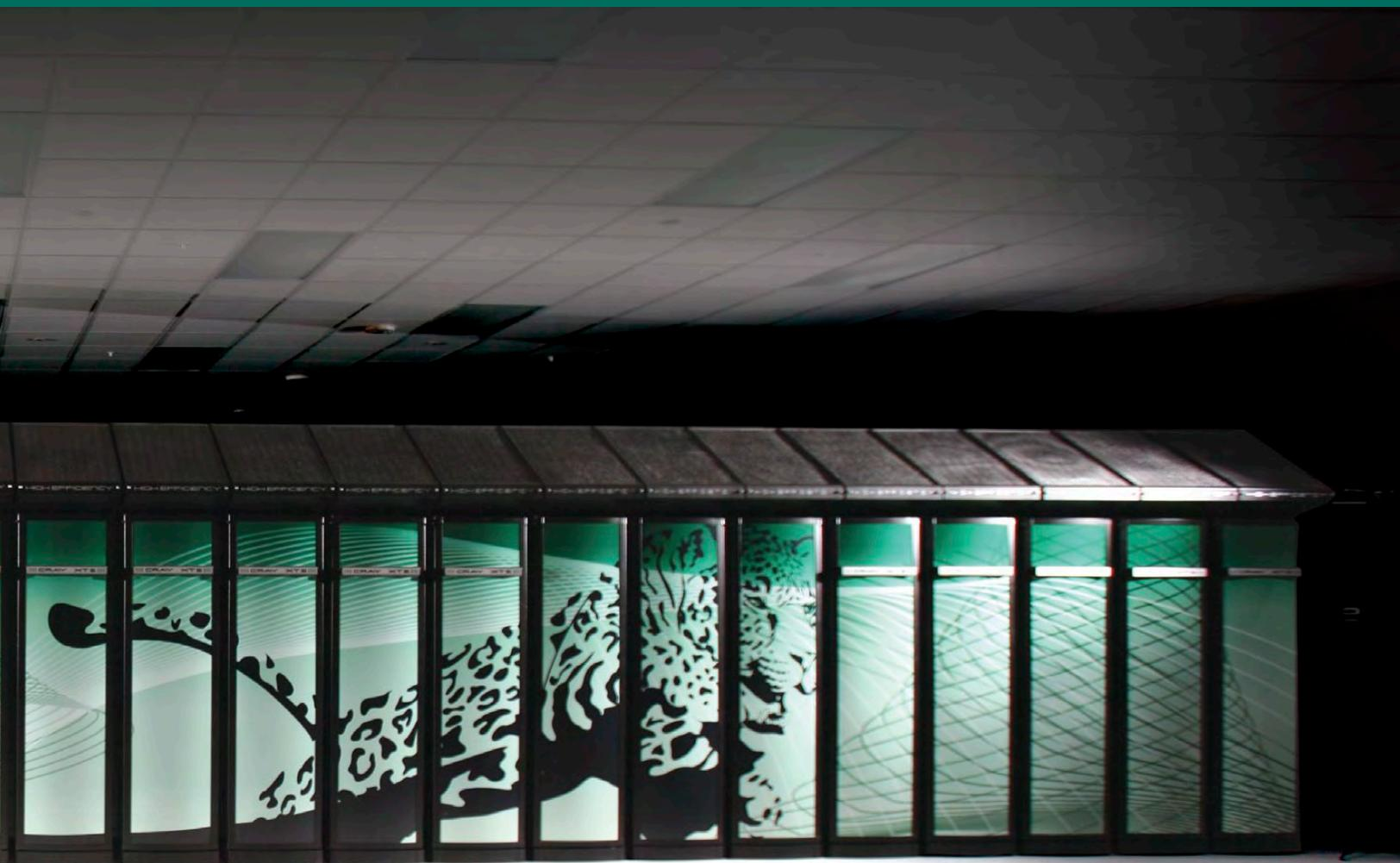
*The new 1.64-petaflop Cray XT Jaguar features more than 180,000 processing cores, each with 2 gigabytes of local memory. The resources of the ORNL computing complex provide scientists with a total performance of 2.5 petaflops.*
