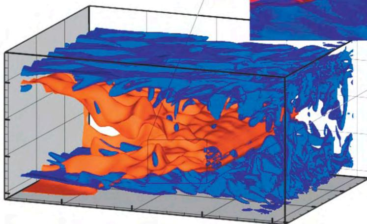
computing facility) we would be simulating incomplete physics: either 2D unsteady flows with detailed chemistry, or 3D turbulent flow with global 1-step chemistry. LCF enables us to include both 3D turbulence and complex chemistry and therefore lets us study turbulence-chemistry interactions in combustion directly.”
