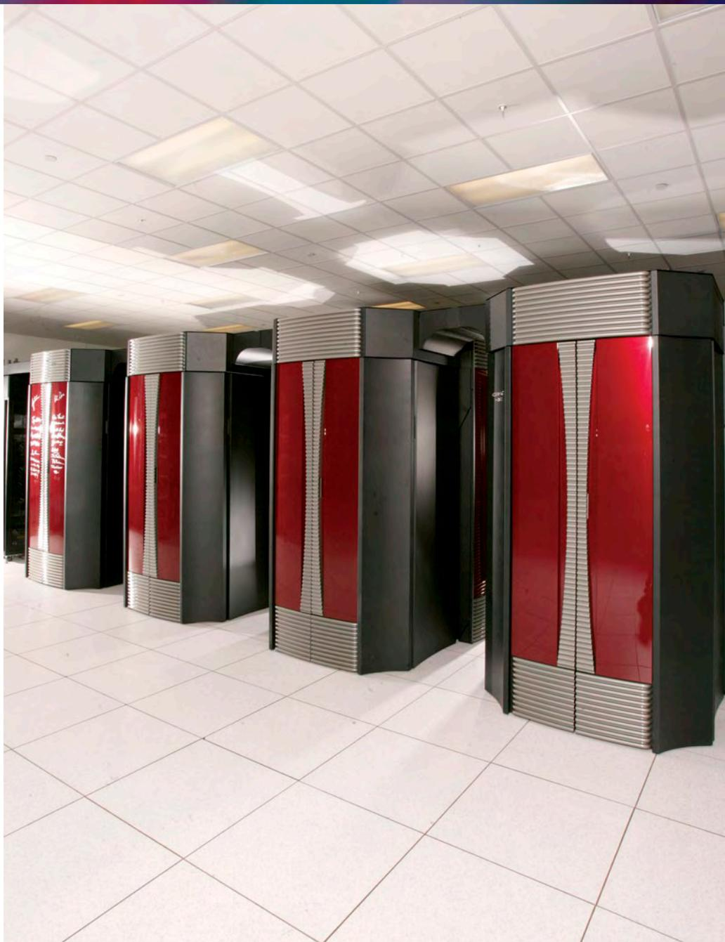
Each MSP has 2 MB of cache. Four MSPs form a node with 8 GB of shared memory. Each MSP contains four single-streaming vector processors with hardware features that allow them to be operated collectively with a second, low-latency level of parallelism called streaming. The compilers can recognize and schedule standard Fortran, C, or C++ code to take advantage of both vectorization and stream parallelism.
