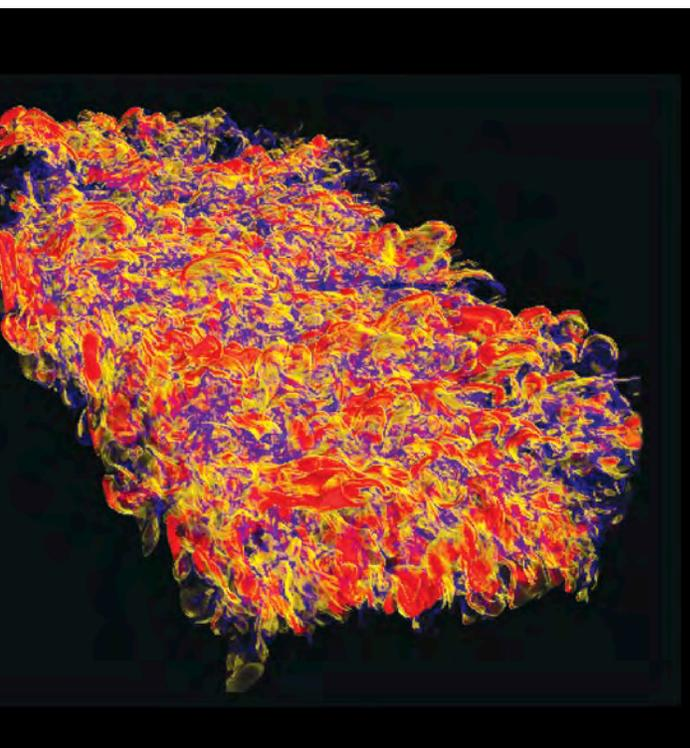
*Simulated planar jet flame, colored by the rate of molecular mixing*
