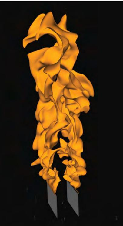
*Direct numerical simulation of a methane-air turbulent Bunsen flame*
