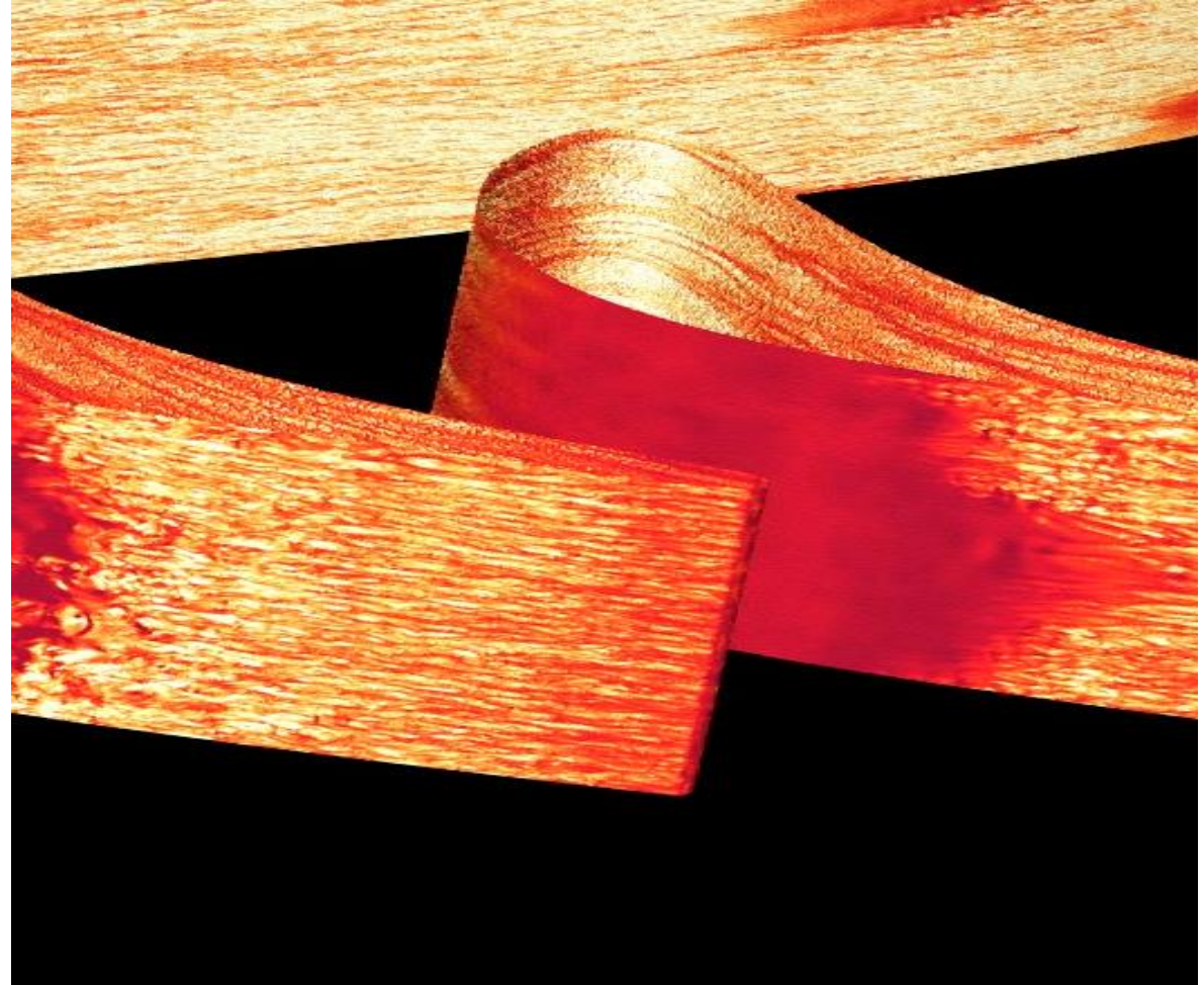
Isosurface of heat flux simulated using 14.6 billion cells.
