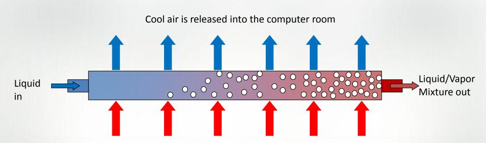
Hot air stream passes through evaporator, rejects heat to R134a via liquid-vapor phase change (evaporation).
