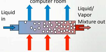
Hot air stream passes through evaporator, rejects heat to R134a via liquid-vapor phase change (evaporation).
